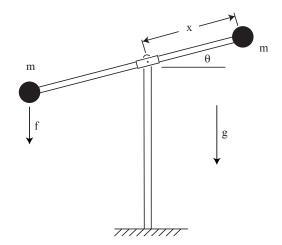
The rod joining the two masses slides frictionlessly in the collar, which pivots frictionlessly; an internal linear spring of stiffness k N/m provides a restoring force to center the rod with respect to the collar. The rod joining the masses is two meters long and x and  $\theta$  are expressed in meters and radians/s.
