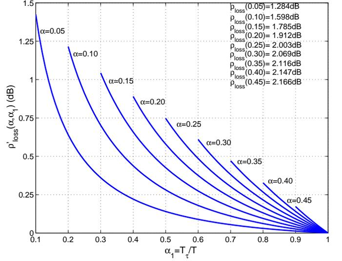
Fig. 4: Asymptotic SNR loss  $\rho'(\alpha, \alpha_1)$  for  $2\alpha \leq \alpha_1 \leq 1$  Fig. 5: Asymptotic SNR loss  $\rho'(\alpha, \alpha_1)$  for  $2\alpha \leq \alpha_1 \leq 1$
