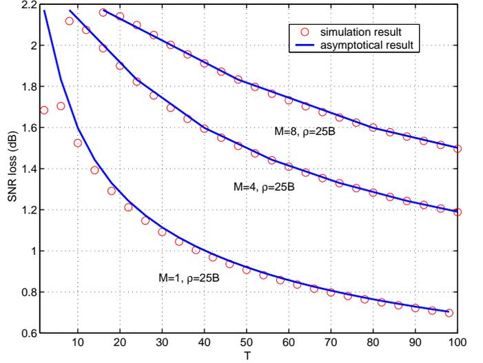
Fig. 2: SNR loss for finite  $\rho$ ,  $M$  and  $T$
