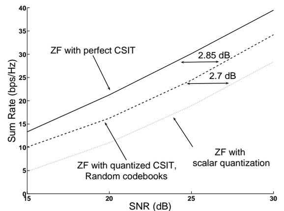
**Fig. 2.** Scalar quantization in MISO systems ( $M = 6, N = 1$ )
