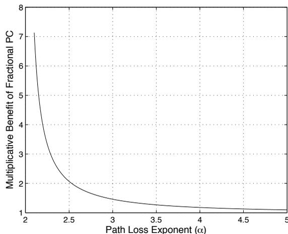
Fig. 3. The ratio of transmission capacity for fractional power control ( $s = \frac{1}{2}$ ) relative to no power control or channel inversion. The gain from FPC becomes quite significant as  $\alpha \rightarrow 2$ .
