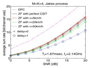
Fig. 3. Rates with feedback delay and Jakes' correlation.
