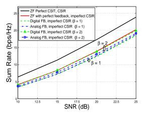
Fig. 1. Quantized vs. Analog Feedback with Imperfect CSIR.
