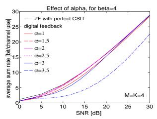
Fig. 2. Quantized feedback with QAM modulation.
