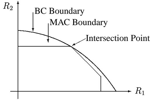
Figure 2: Capacity regions for a constant MAC and its dual BC with  $h_1 > h_2$ .
