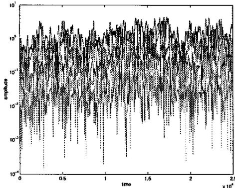
Fig. 5. A specific realization of random process defined by five Rayleigh fading channel taps ( $\alpha = 0$ ).
