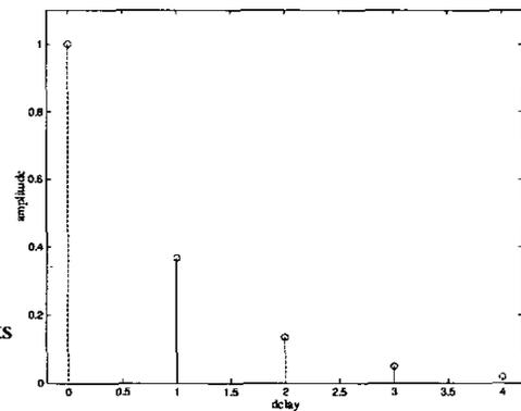
Fig. 4. Exponential power-delay profile (5 taps).
