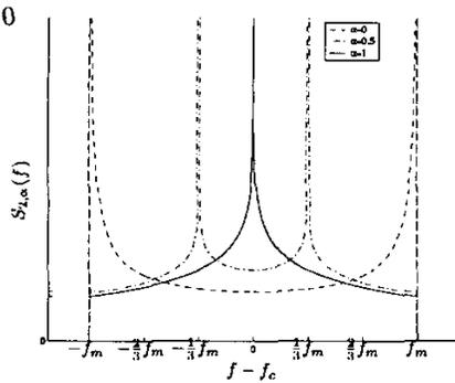
Fig. 2. Rayleigh Doppler Spectrum: Ad hoc Case, Fixed  $f_m$
