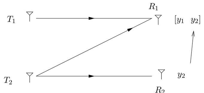
Fig. 4. The “Z<sub>upper</sub>” Channel
