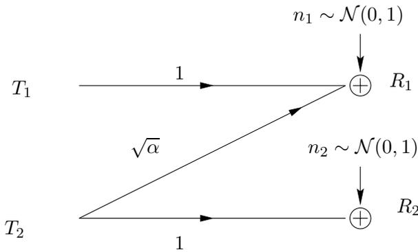
Fig. 2. The Gaussian “Z” Channel
