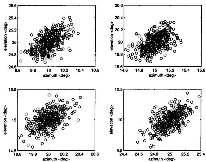
Fig. 5. Azimuth-elevation scatter zoom-in, SNR = 12 dB.
