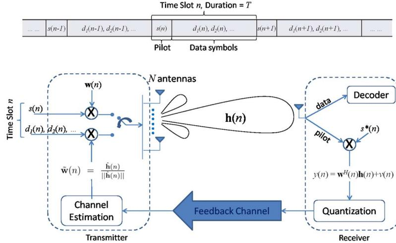
Fig. 1. Downlink frame structure and limited feedback beamforming system model.
