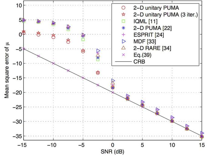
Fig. 3. MSE of  $\mu$  versus SNR. ( $M = N = 5$ ,  $\mu = -0.12\pi$  and  $\nu = 0.2\pi$ ).
