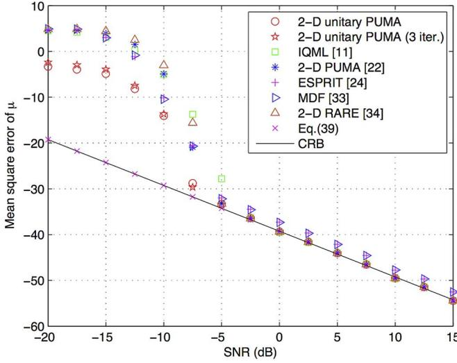
Fig. 1. MSE of  $\mu$  versus SNR. ( $M = N = 15$ ,  $\mu = -0.12\pi$  and  $\nu = 0.2\pi$ ).
