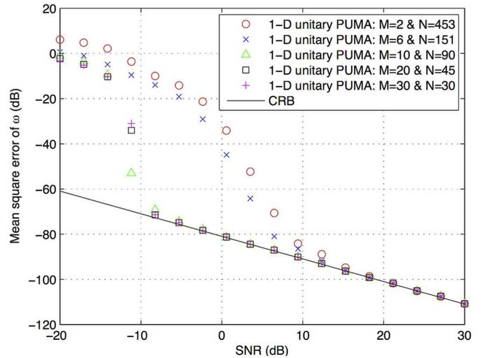
Fig. 7. MSE of  $\omega$  versus SNR. ( $L = 907$ ,  $\omega = 0.2\pi$  and  $\bar{\kappa} = e^{j1}$ ).
