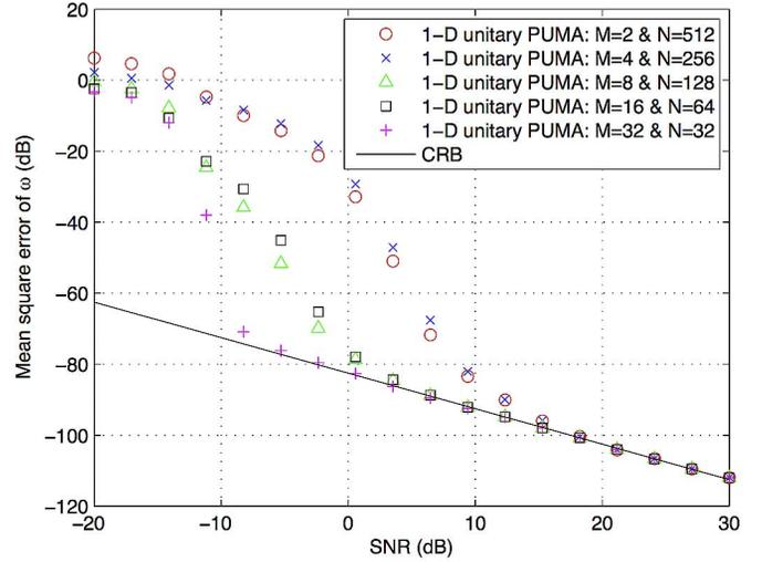
Fig. 6. MSE of  $\omega$  versus SNR. ( $L = 1024$ ,  $\omega = 0.2\pi$  and  $\bar{\kappa} = e^{j1}$ ).
