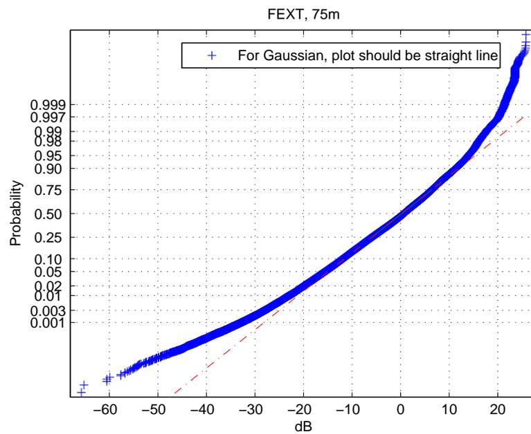
Fig. 5. Deviation from Gaussian p.d.f for FEXT, 75m
