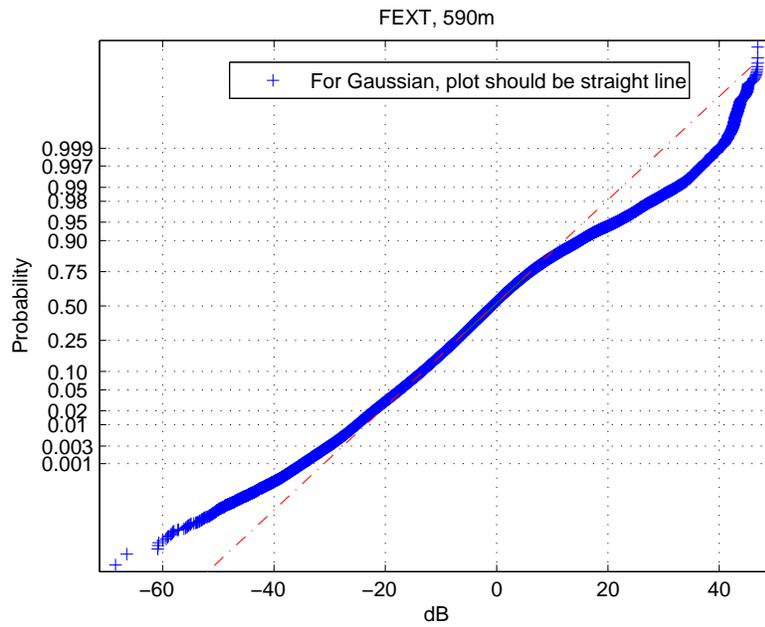
Fig. 11. Deviation from Gaussian p.d.f for FEXT, 590m
