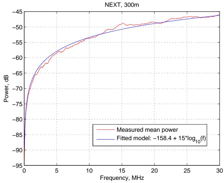
Fig. 1. Measured mean power and fitted model for NEXT, 300m (mean std = 9.5dB)
