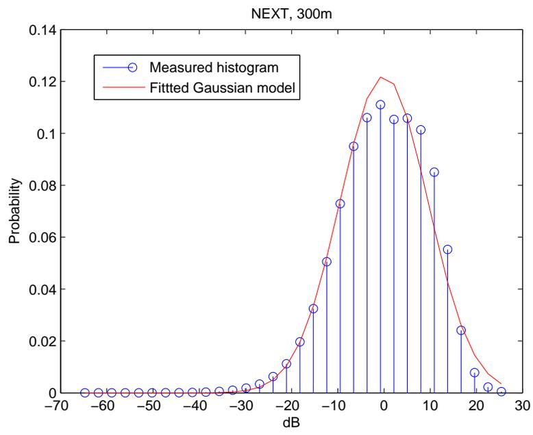
Fig. 3. Histogram of the mean-centered power for NEXT, 300m
