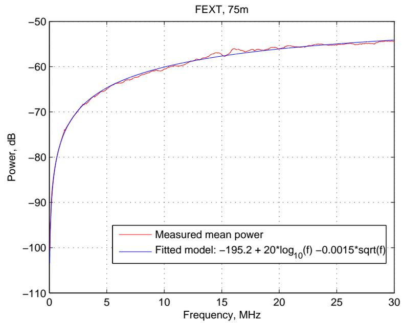
Fig. 4. Measured mean power and fitted model for FEXT, 75m (mean std = 9dB)
