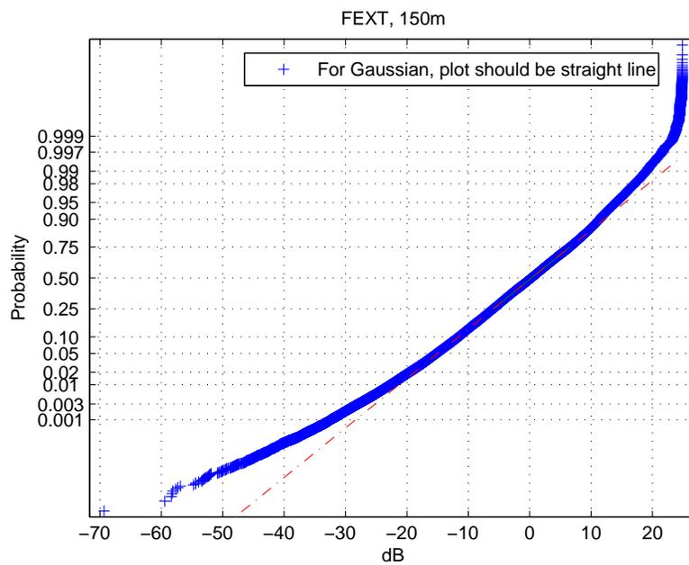
Fig. 7. Deviation from Gaussian p.d.f for FEXT, 150m
