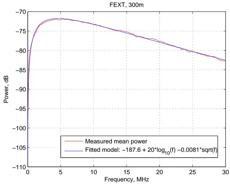
Fig. 8. Measured mean power and fitted model for FEXT, 300m (mean std = 8.8dB)
