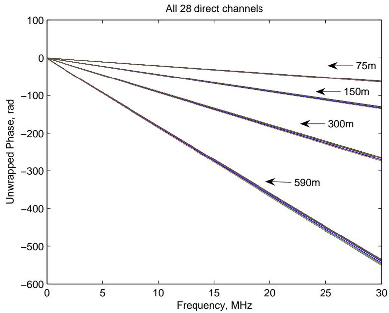
Fig. 15. Unwrapped phase of direct channels
