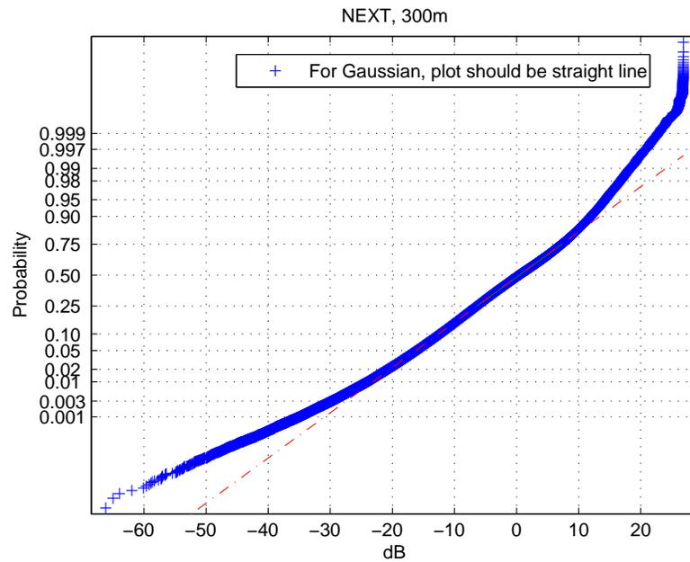
Fig. 2. Deviation from Gaussian p.d.f for NEXT, 300m
