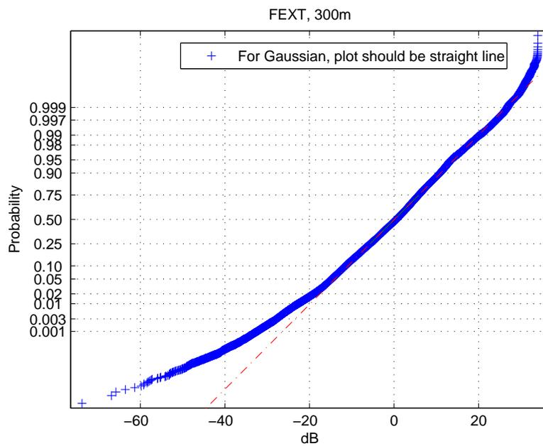
Fig. 9. Deviation from Gaussian p.d.f for FEXT, 300m
