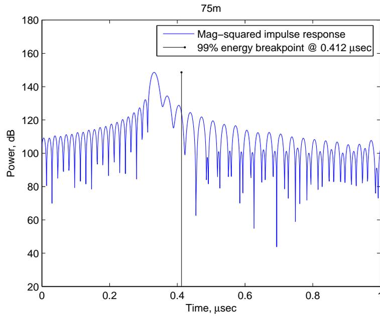
Fig. 16. Magnitude squared of direct channel's impulse response, 75m
