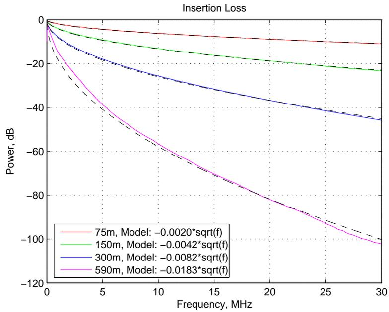
Fig. 14. Measured mean power of direct channel and fitted model
