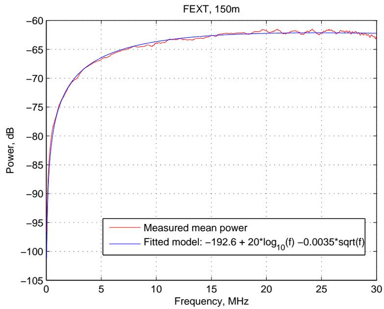
Fig. 6. Measured mean power and fitted model for FEXT, 150m (mean std = 9dB)
