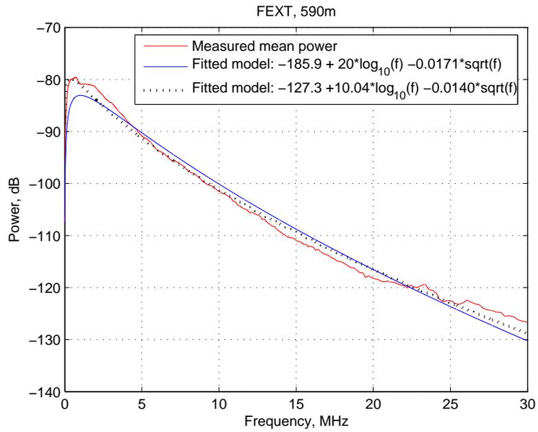
Fig. 10. Measured mean power and fitted model for FEXT, 590m (mean std = 11.2dB)
