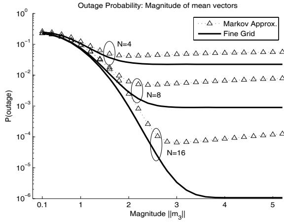
Fig. 6. Magnitude of mean vectors( $J = 3$ ): Outage Probability as a function of the magnitude:  $\mathcal{M}(\mathbf{w}_{opt})$  and  $\mathcal{M}(\mathbf{w}_{apr})$  versus  $\|\mathbf{m}_3\|$ .
