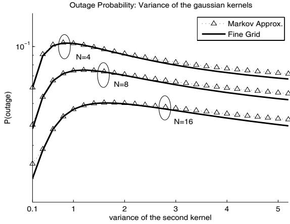
Fig. 11. Variance of the Gaussian Kernels: Outage Probability as a function of the variance:  $C(\mathbf{w}_{opt})$  and  $C(\mathbf{w}_{apr})$  versus  $\sigma_2^2$ .
