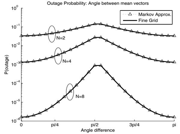
Fig. 1. Angle between mean vectors ( $J = 2$ ): Outage Probability as a function of the angle:  $\mathcal{M}(\mathbf{w}_{opt})$  and  $\mathcal{M}(\mathbf{w}_{app})$  versus  $\hat{\phi}$ .
