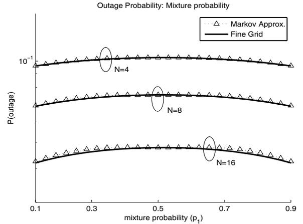
Fig. 12. Mixture Probability: Outage Probability as a function of the mixture probability:  $\mathcal{C}(\mathbf{w}_{opt})$  and  $\mathcal{C}(\mathbf{w}_{appr})$  versus  $p_1$ .
