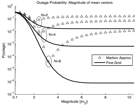
Fig. 2. Magnitude of mean vectors( $J = 2$ ): Outage Probability as a function of the magnitude:  $\mathcal{M}(\mathbf{w}_{opt})$  and  $\mathcal{M}(\mathbf{w}_{apr})$  versus  $\|\mathbf{m}_2\|$ .
