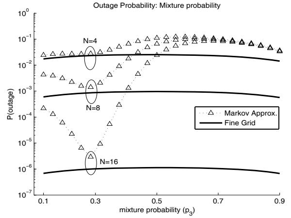
Fig. 8. Mixture Probability( $J = 3$ ): Outage Probability as a function of the mixture probability:  $\mathcal{M}(\mathbf{w}_{opt})$  and  $\mathcal{M}(\mathbf{w}_{apr})$  versus  $p_3$ .
