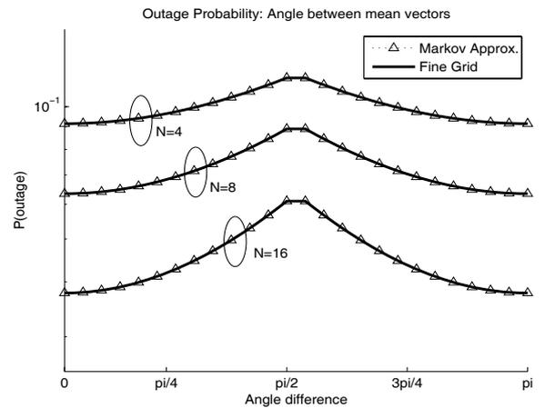
Fig. 9. Angle between mean vectors: Outage Probability as a function of the angle:  $\mathcal{C}(\mathbf{w}_{opt})$  and  $\mathcal{C}(\mathbf{w}_{apr})$  versus  $\theta$ .
