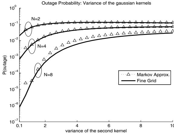
Fig. 3. Variance of the Gaussian Kernels( $J = 2$ ): Outage Probability as a function of the variance:  $\mathcal{M}(\mathbf{w}_{opt})$  and  $\mathcal{M}(\mathbf{w}_{apr})$  versus  $\sigma_2^2$ .
