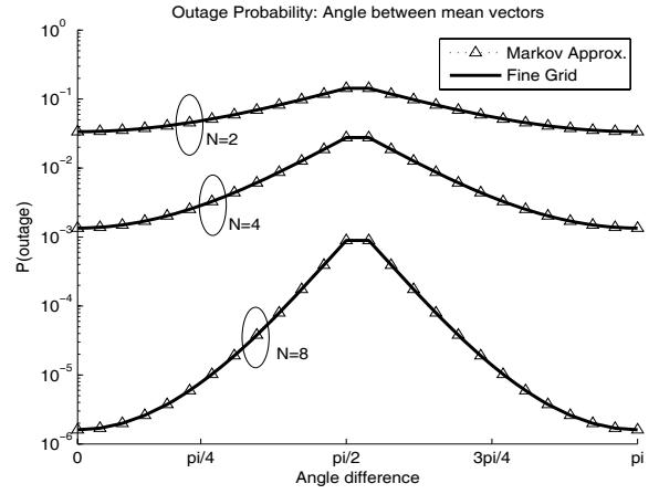
Fig. 1. Angle between mean vectors ( $J = 2$ ): Outage Probability as a function of the angle:  $\mathcal{M}(\mathbf{w}_{opt})$  and  $\mathcal{M}(\mathbf{w}_{apr})$  versus  $\hat{\phi}$ .
