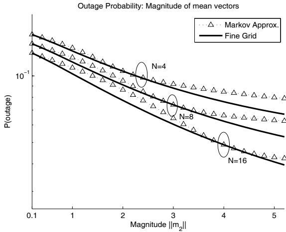
Fig. 10. Magnitude of mean vectors: Outage Probability as a function of the magnitude:  $C(\mathbf{w}_{opt})$  and  $C(\mathbf{w}_{apr})$  versus  $\|\mathbf{m}_2\|$ .
