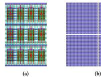
Figure 4: Parameterized primitive layouts for (a) a differential pair with transistors placed using common centroid, and (b) a  $2 \times 2$  MOM capacitor array.
