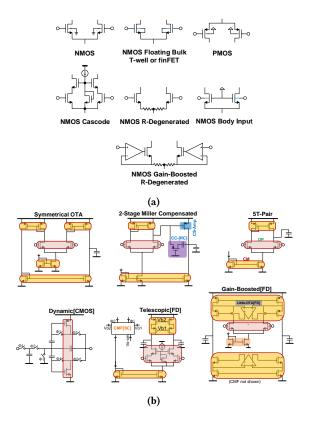
Figure 3: Example variants of (a) the differential pair (DP) primitive (b) the opamp/OTA, showing fundamental primitives.
