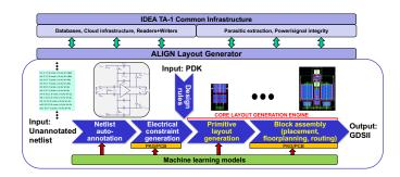
Figure 1: Overview of the ALIGN flow.
