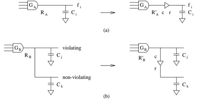
Figure 2. Buffer Insertion (a) Type A (b) Type B
