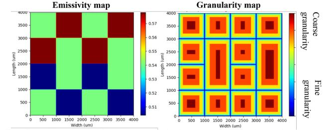
Fig. 7. Adaptive gridding strategy which maintains a high resolution (small element sizes) in the die regions with emissivity gradients. The testcase from [13] with four different element sizes.
