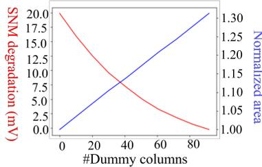
Fig. 11. Area and SNM tradeoff due to insertion of dummy columns.
