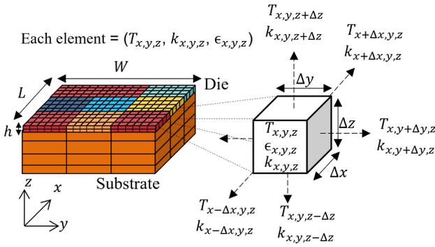
Fig. 4. FDM-based spatial derivative estimation.
