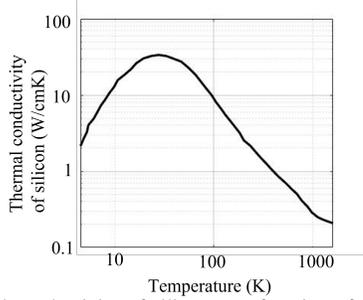
Fig. 5. Thermal conductivity of silicon as a function of temperature [12].
