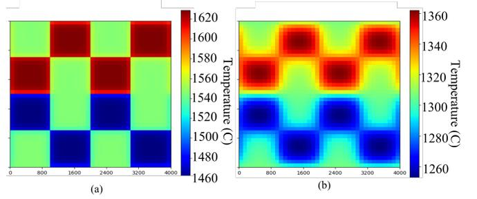
Fig. 6. Thermal profile of the testcase from [13] with a checkerboard pattern of emissivity (a) with and (b) without considering the dependence of the thermal conductivity of silicon on temperature. A lamp temperature of 1800°C and pulse time of 5ms is used.
