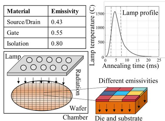
Fig. 1. RTA process highlighting wafer heating through radiation, the temperature profile of the lamp with millisecond anneal times and a 5ms pulse, and intra-die emissivity pattern variations.
