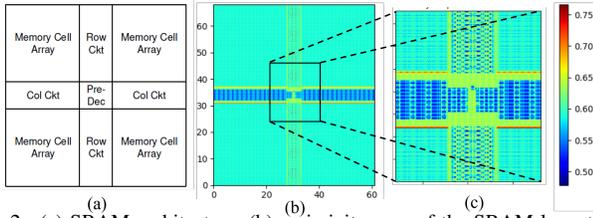
Fig. 2. (a) SRAM architecture, (b) emissivity map of the SRAM layout, and (c) zoomed-in version of the layout showing variation in emissivity differences between array and peripheral circuitry.
