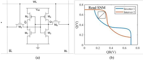
Fig. 3. (a) SRAM 6T cell and (b) butterfly curve for read SNM calculation.
