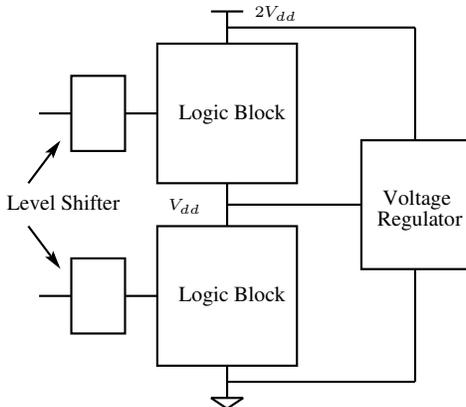
Figure 6: A schematic of a 2-level stacked- $V_{dd}$  circuit structure.
