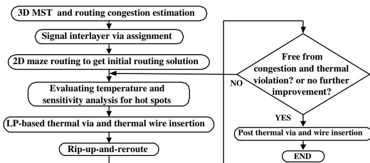
Figure 3: Overall flow for the temperature-aware 3D global routing algorithm.
