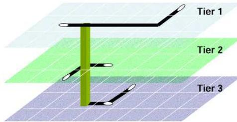
Figure 2: An example route for a net in a three-tier 3D technology.
