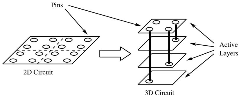
Figure 5: Power pin limitations for a 3D chip, as compared to a 2D chip with the same amount of circuitry.
