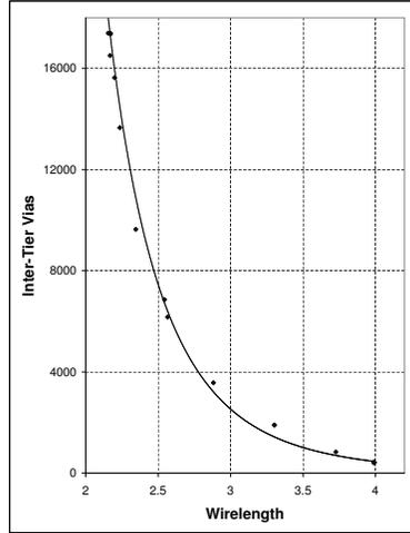
Figure 1: Tradeoff between the number of interlayer vias versus the total wire length for the benchmark ibm01
