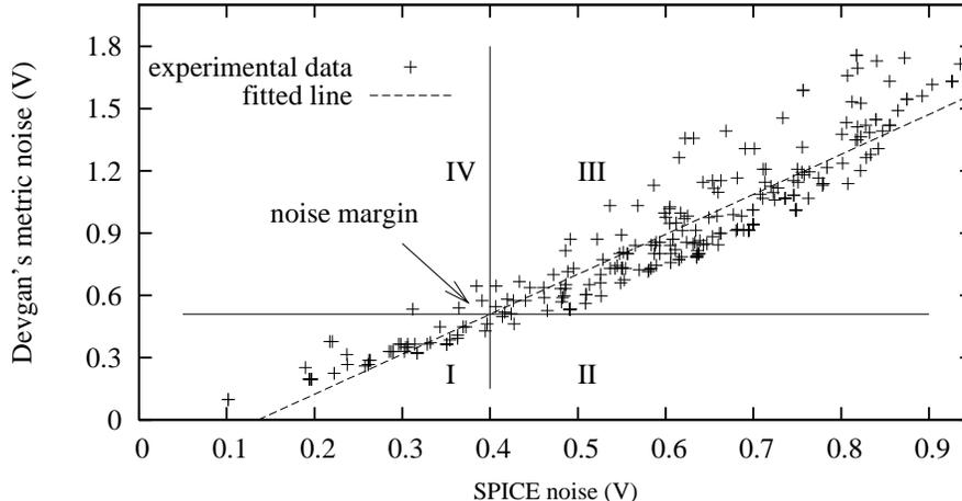
Fig. 4. Noise estimation under Devgan's metric and SPICE simulation. The least squares fit to a linear approximation between the two noise metrics is drawn as a dashed line. The plane is divided into four representative regions, I through IV, as shown above.
