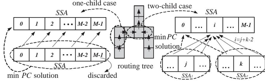
Fig. 7. Updating SSA for one-child and two-child grid cells.
