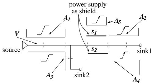
Fig. 2. Switching noise on a victim net with shielding supply wires.  $V$  is the victim net,  $A_i$ ,  $i = 1, \dots, 5$  are potential aggressor nets, and  $s_1, s_2$  are power supply shields.
