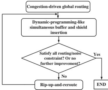
Fig. 5. Overall flow of global routing with simultaneous shield and buffer insertion for crosstalk noise reduction.
