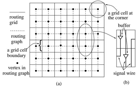
Fig. 1. Routing grid and buffer insertion for signal wires.
