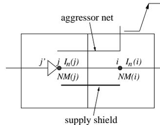
Fig. 3. Calculation of noise margin by Devgan's metric.
