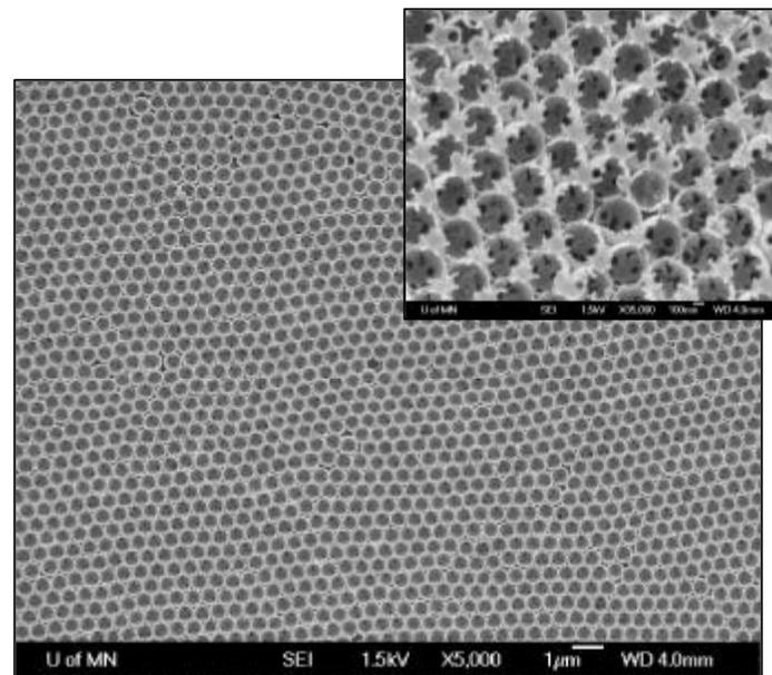
Inverse Opals composed of tin-oxide nanoshells, 10-30 nm thick
