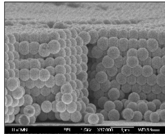
Tin oxide infiltrated spheres
