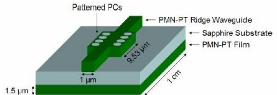
A ridge waveguide will couple light to a structure in the middle of the sample, where photonic crystals will be patterned. This configuration will be used to demonstrate optical waveguides, switches, filters and other integrated photonic devices.
