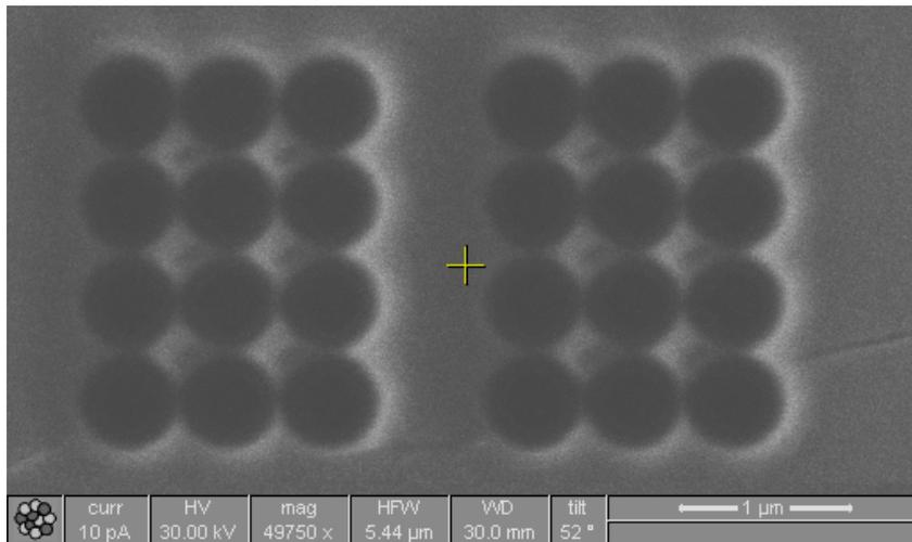
Photonic crystal air holes (circles) and defect (column between circles) patterned using a Focused Ion Beam. The nanometer resolution of this equipment allows the realization of arbitrary patterns.
